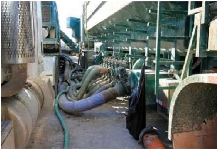
To generate sand slurry requires a low-pressure manifold to mix water and polymers with sand. Credit: Tadeusz Patzek
